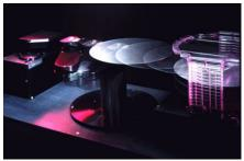
Cassette-to-cassette robotic handling provides completely automated measurement
